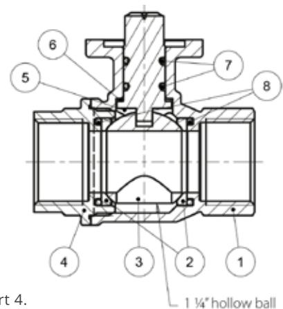
DN shows the nominal flow diameter. Actual flow diameter complies with full port DIN 3357 part 4.
