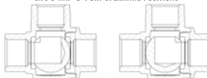
S.76 3-WAY "L" PORT OPERATING POSITIONS
