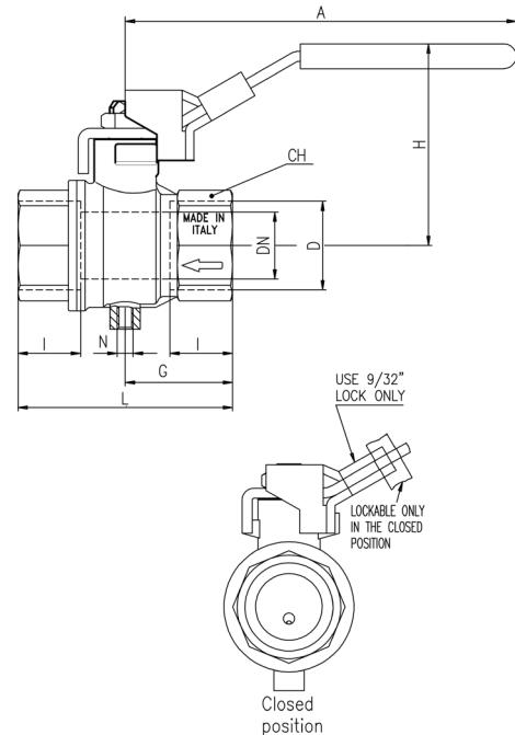
DN shows the nominal flow diameter. Actual flow diameter complies with full port DIN 3357 part 4.
