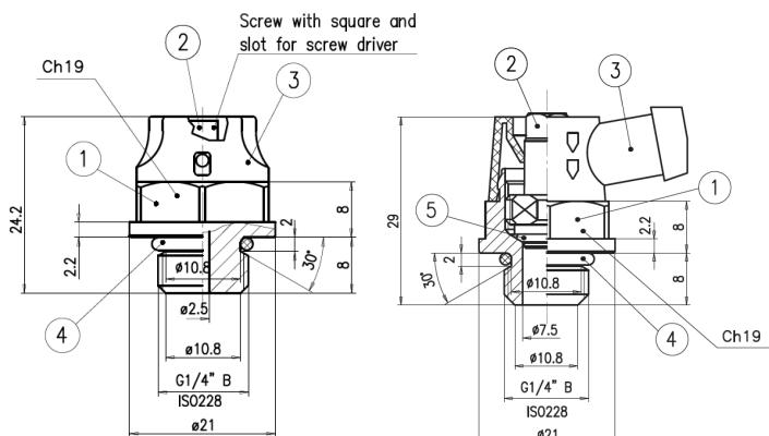
PSPR81 - Side drain valve G 1/4" with hose connection
