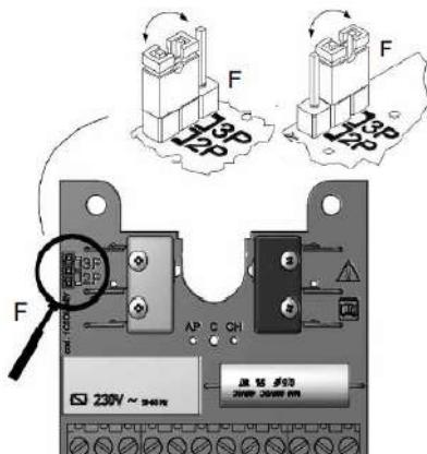
**Vac models:** Move the jumper to have the desired electrical connection.
