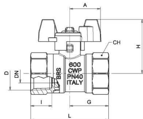
DN shows the nominal flow diameter. Ball valves are marked CE on handle from 1 1/2" to 2" as follow:
