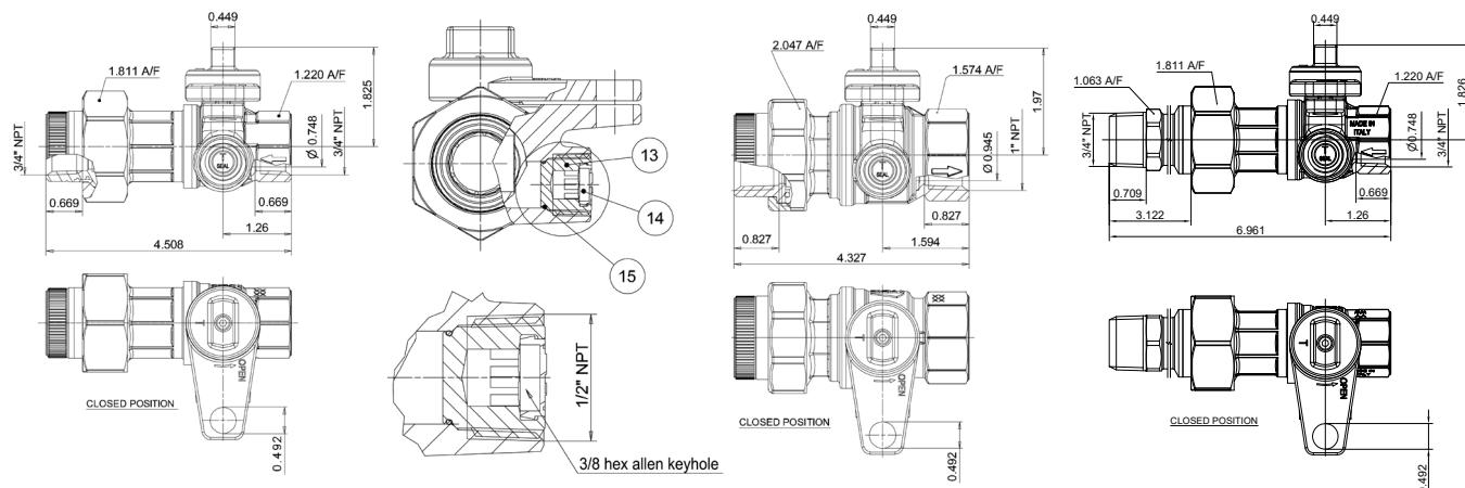
DN shows the nominal flow diameter. Actual flow diameter complies with full port DIN 3357 part 4.
