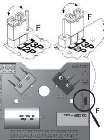
**Vac models:** Move the jumper to have the desired electrical connection.
