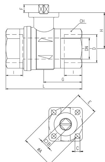
Ball valves are marked CE on end-cap from 1 1/4" to 4" as follow: CE 0425 cat IIIB+D PS: 5 GAS TS1:-20°C TS2:+60°C
