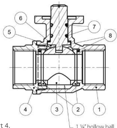
DN shows the nominal flow diameter. Actual flow diameter complies with full port DIN 3357 part 4. Ball valves s.65 size 1 1/4" are marked CE as follows: CE Cat I-A
