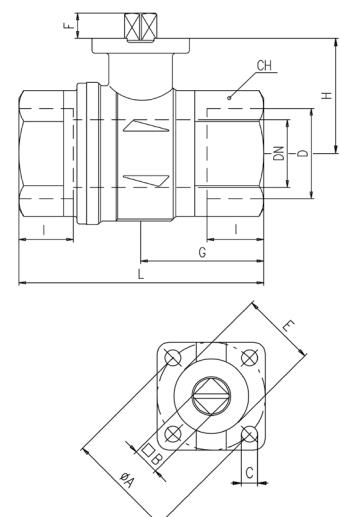
Ball valves are marked CE on end-cap from 1 1/4" to 4" as follow: CE 0425 cat IIIB+D PS: 5 GAS TS1:-20°C TS2:+60°C
