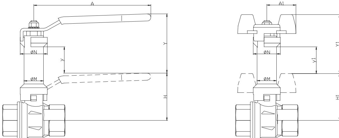
Dimensions Y, y, Y1 and y1 are additional to dimension H on the relevant valve drawing
