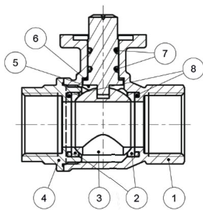
DN shows the nominal flow diameter. Actual flow diameter complies with full port DIN 3357 part 4.
