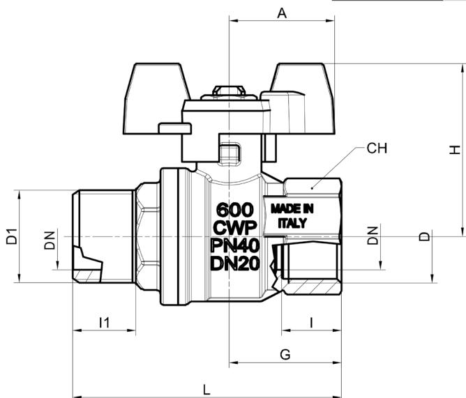
DN shows the nominal flow diameter. Actual flow diameter complies with full port DIN 3357 part 4.
