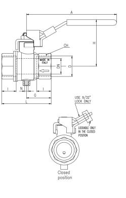
DN shows the nominal flow diameter. Actual flow diameter complies with full port DIN 3357 part 4.
