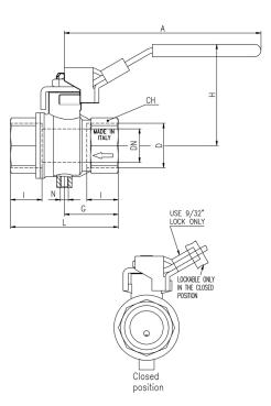
DN shows the nominal flow diameter. Actual flow diameter complies with full port DIN 3357 part 4.
