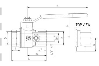
$\,$  DN shows the nominal flow diameter. Actual flow diameter complies with full port DIN 3357 part 4.
