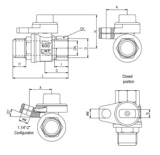
DN shows the nominal flow diameter. Actual flow diameter complies with full port DIN 3357 part 4.
