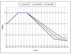
The given data of the pressure-temperature chart refer to the valve body
