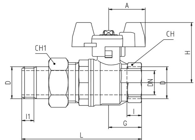
DN show the nominal flow diameter. Actual flow diameter complies with full port DIN 3357 part 4.
