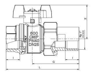
DN shows the nominal flow diameter. Actual flow diameter complies with full port DIN 3357 part 4.
