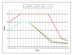
AS4617 limitations for GAS: 2100 Kpa up to 2" and 1500 Kpa from 2  $\frac{1}{2}$ " to 4" rated working pressure and 0°C +60°C temperature
