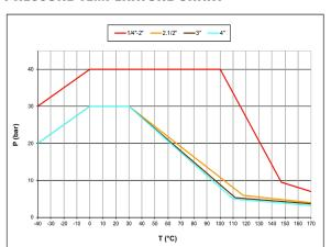
AS4617 limitations for GAS: 2100 Kpa up to 2" and 1500 Kpa from 2  $\frac{1}{2}$ " to 4" rated working pressure and 0°C +60°C temperature
