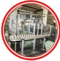
Automatic valve assembly and testing equipment 1/8" thru 4"
