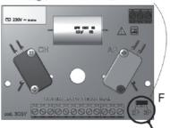
**Vac models:** Move the jumper to have the desired electrical connection.
