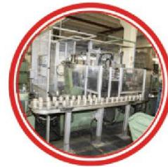
Automatic valve assembly and testing equipment 1/8" thru 4"
