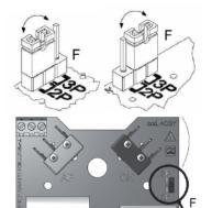
**Vac models:** Move the jumper to have the desired electrical connection.
