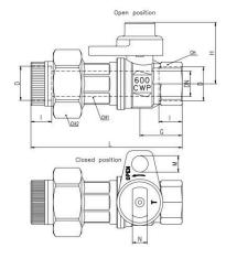
DN shows the nominal flow diameter. Actual flow diameter complies with full port DIN 3357 part 4.  $\,$
