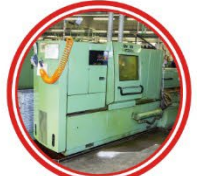
6-spindle and 8-spindle lathe machines with automatic loaders
