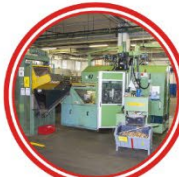
Transfer machines for forgings with automatic loaders
