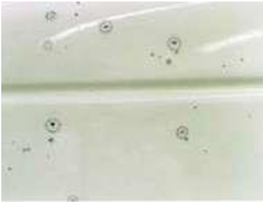
Small, crater-like openings in the finish caused by contamination on the surface being painted
